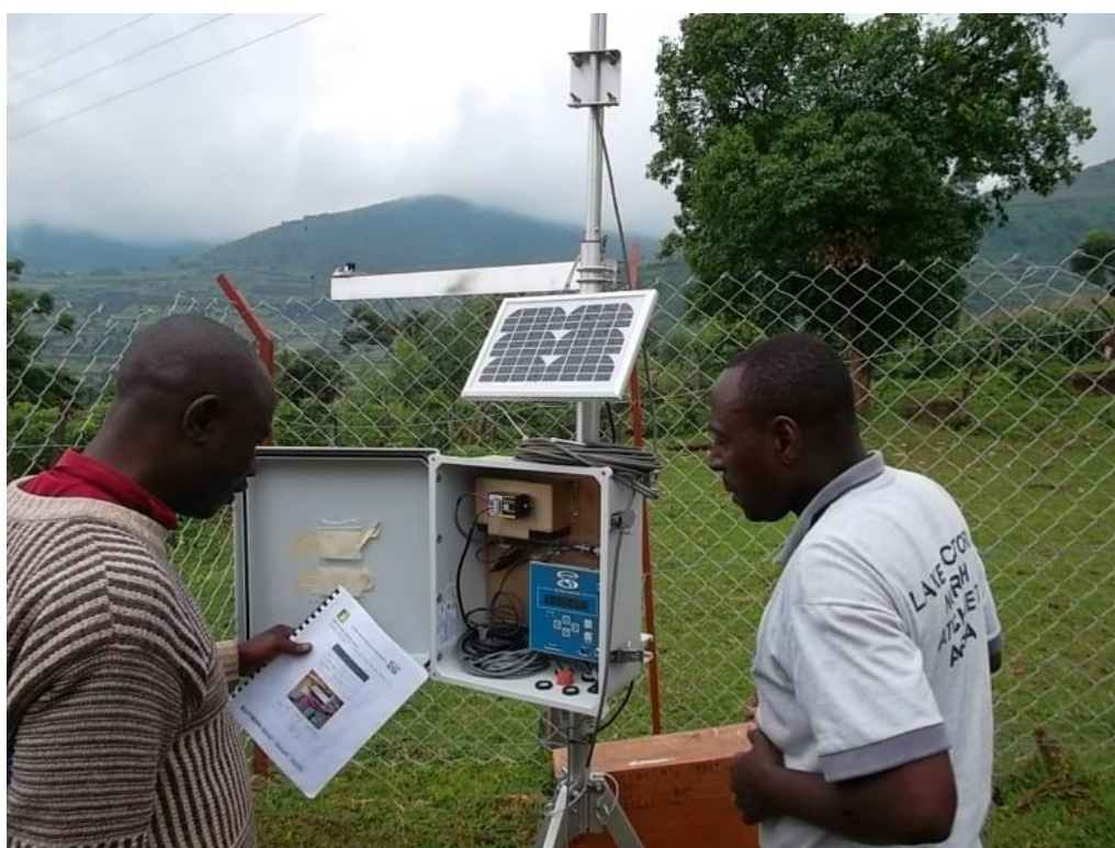
Figure 4: Technical Officers from LVNCA taking readings from an automatic weather station at Bumbale installed by the SMM Project (SMM, 2011).
